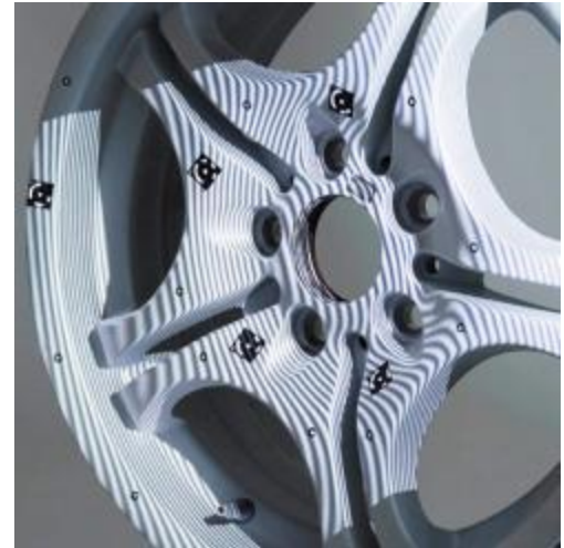
Figure 96: Structured Light Pattern Designed for Surface Inspection
