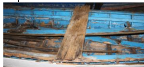
Figure 46: Picture of a boat considered to be repairable, but not floatable
