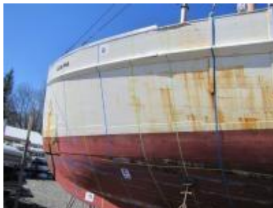
Figure 52: The Jacob Pike prepared for taking pictures for photogrammetry
