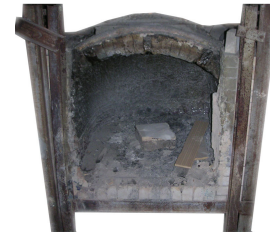
Figure 8: Traditional Murano Furnace with Front Wall Removed for Servicing
