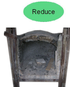
Figure 13: Traditional Murano Furnace with Front Wall Removed for Servicing
