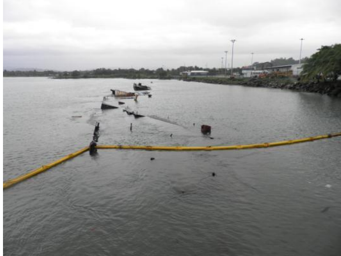
Figure 12: Floating boom in Port of Limón surrounding part, but not all of a submerged vessel (Hayley Sandgren, 2011)
