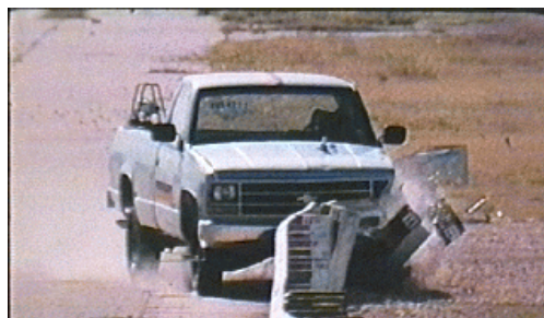
Figure 4.43: Sequential frontal views of impact event - TTI test 405421-1 and F.E. analysis.
