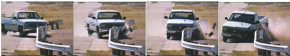
Figure 4.4: TTI test 405421-1 on the modified G4(1S) with wood blockouts.(57)
