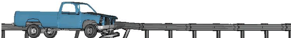
Figure 4.44: Sequential oblique views of impact event - TTI test 405421-1 and F.E. analysis.
