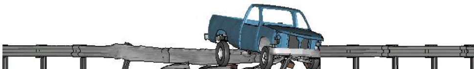
Figure 4.44: (CONTINUED) Sequential oblique views of impact event - TTI test 405421-1 and F.E. analysis.
