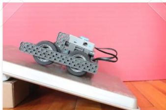
Inclined Plane: an inclined plane is a surface that is placed at an angle. This angle can help someone get from a low place to a high place easier, like the robot in the picture!
