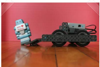
Wedge: a wedge is similar to an inclined plane, but instead this angled surface is used to push objects, like how the VEX robot is pushing the WPI robot!
