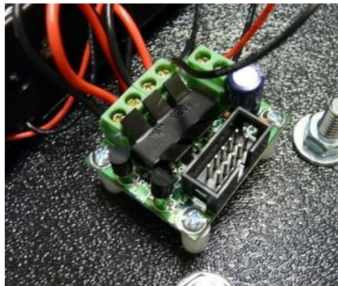
Figure 12 - WIRZ #203 Motor Controller Mounted to Robot Deck
