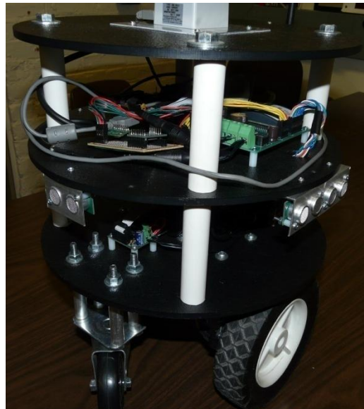
Figure 19 - Robot Base with Ultrasonic Sensor Array
