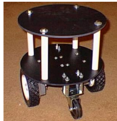
Figure 5 - Max '99 Robot Base. Adapted from Zagros robotics website. ( https://www.zagrosrobotics.com/show/item.asp?itemid=523 )
