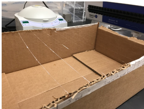
Figure 20: Drying of the Microthreads with warm air at a medium fan speed
