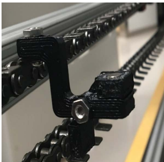
Figure 49: Clamp made through rapid prototyping in the closed position
