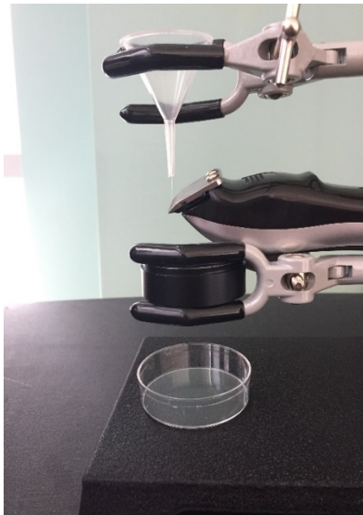
Figure 45: Final Mechanism with the Funnel to Bundle the Fibrin
