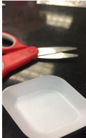
Figure 51: Cutting of Threads into particles using small scissors. Threads cut onto weigh plate for measuring
