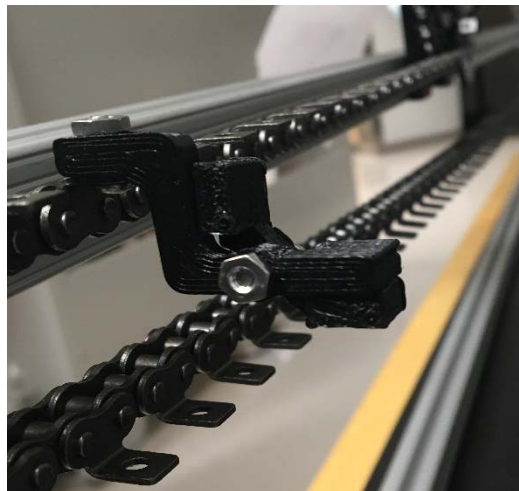
Figure 48: Clamp made through rapid prototyping in the open position
