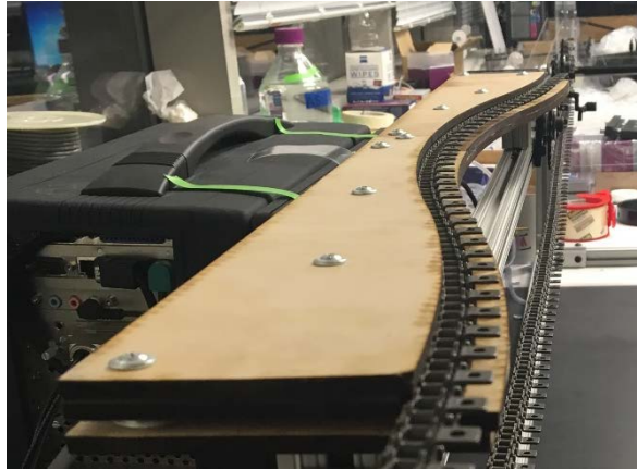
Figure 50: Stretching platform prototype made of birch plywood
