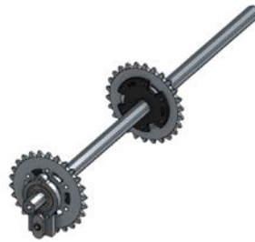
Figure 109: CAD Assembly of Drive Shaft Bearing Assembly, Sprockets, and Hex Bar
