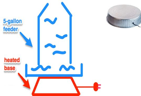
**Figure 12: Heated base setup<sup>2</sup> (left) and Heated base<sup>3</sup> (right)**
