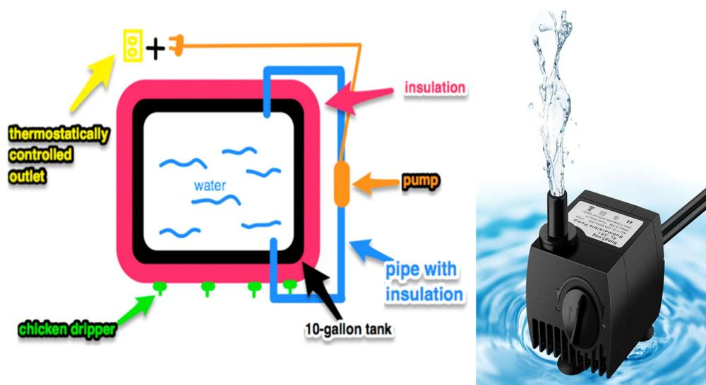
**Figure 13: Insulated pump tank setup<sup>4</sup> (left) and Pump<sup>5</sup> (right)**
