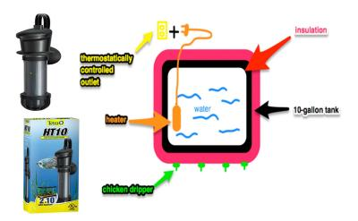
Figure 15: Heater<sup>7</sup> (left) and Insulated heated tank setup<sup>8</sup> (right)
