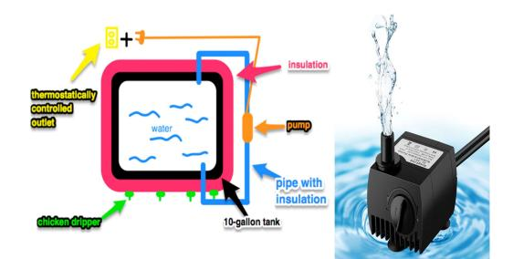
Figure 13: Insulated pump tank setup<sup>4</sup> (left) and Pump<sup>5</sup> (right)
