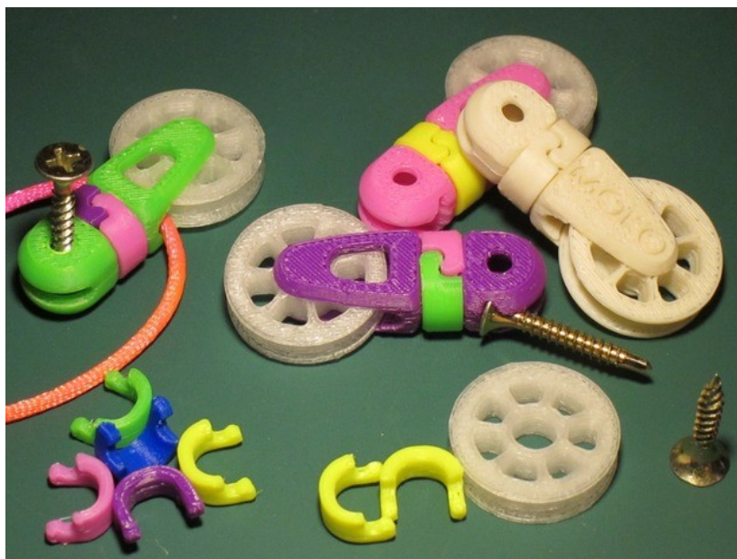
Figure 5. 3D printed pulleys for use in physics classes. www.thingiverse.com 47 by Moko under CC BY 2.0 by Creative Commons
