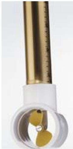
**Figure 53. Plastic Probe Propeller**
