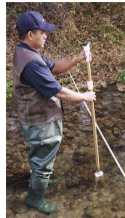
**Figure 54: Proper Positioning of Probe**
