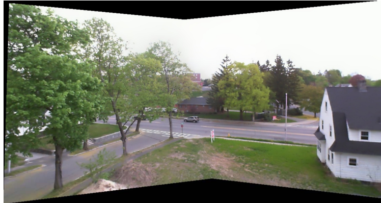
Figure 4.10: Stitching Result with a Planar Compositing Surface
