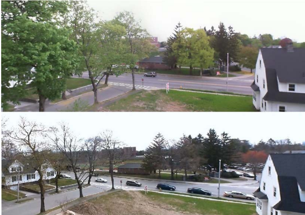
Figure 4.22: Comparison of Panoramas - top: feature-based method, bottom: homography-based method
