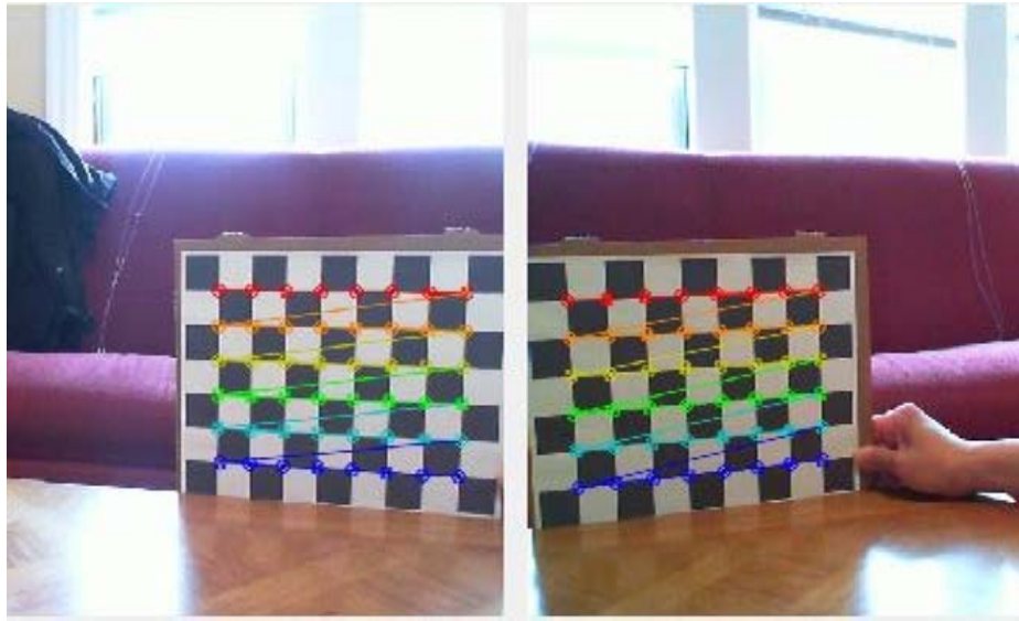
Figure 4.14: Chessboard with Corners Marked by Color Circles and Lines
