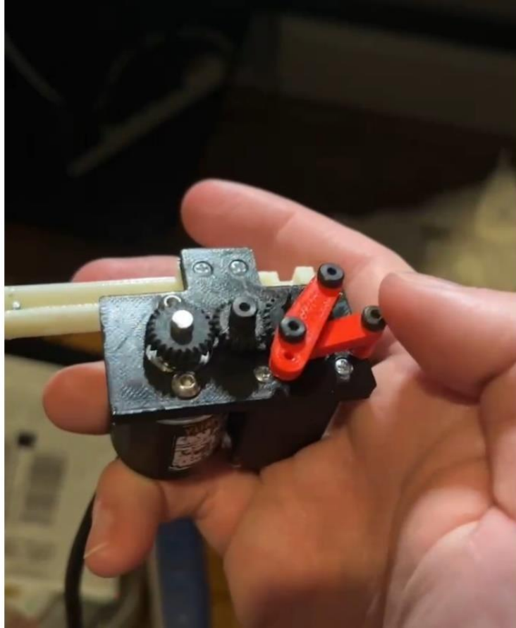
Fig. 3–22: 3D printed well-assembled motor module with encoder design.
