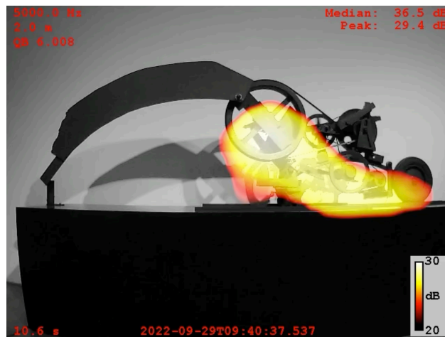
Figure 8: Sample frame of Tinguely's Char M.K. captured from the acoustic camera with an overlaid heatmap of the mechanism's sound intensity at a particular frequency
