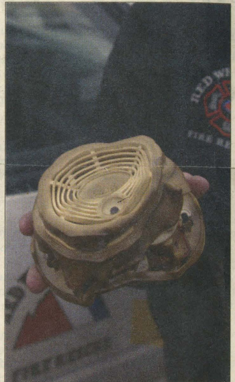
Special to the Daily/Carl Scofield The temperature in a Mill Run condo fire in Warrior's Mark was so hot, it melted the smoke detector into a twisted blob of plastic.
