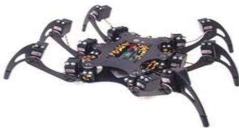
Figure 9 – Phoenix - three degree of freedom legs
