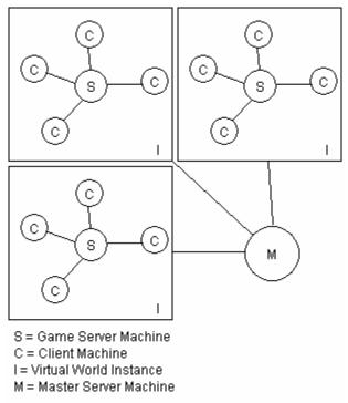
Figure 4-1: Client-server Architecture with Instancing
