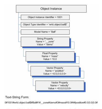
Figure 6.5.6-1: Object Instance Architecture with String Encoding
