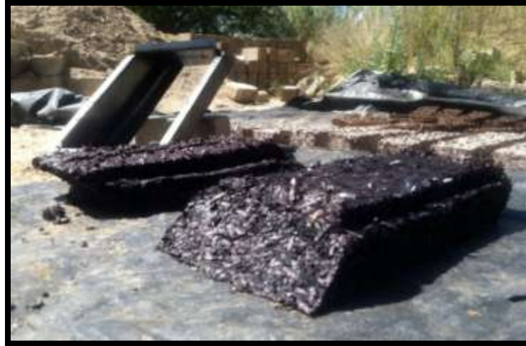
FIGURE 16: PROTOTYPE INSULATION MOLD AND SHEETS 70
