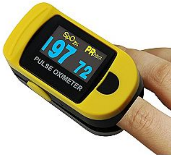
Figure 3.4: Pulse Oximeter - Displaying oxygen saturation level and pulse rate
