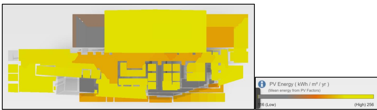
Figure 7.9: Solar Panel Roof Layout with Key
