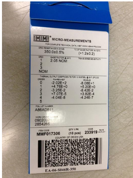
Figure 12: Strain Gage information
