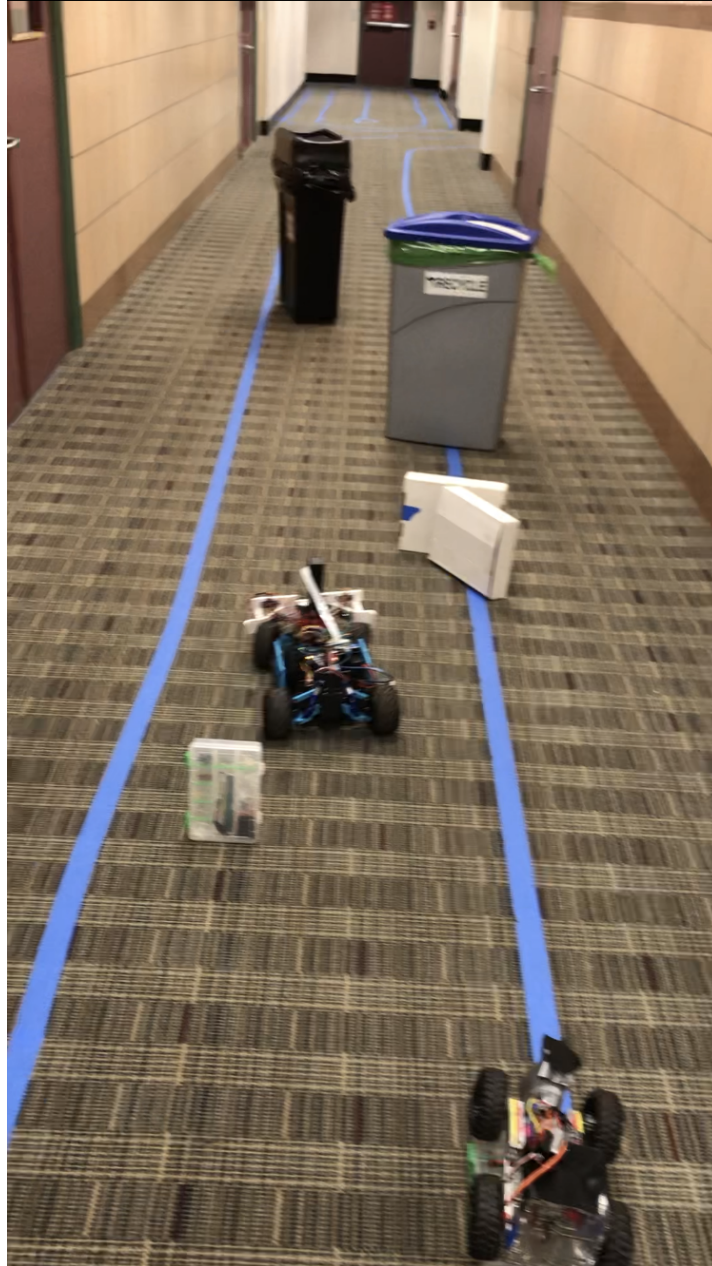
Figure 10.12: Obstacle Avoidance Testing
