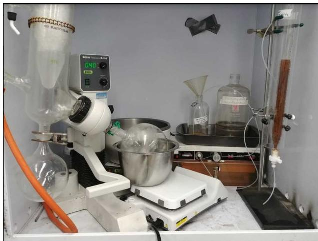
**Figure 5.2.1.** Rotary evaporator hood configuration.
