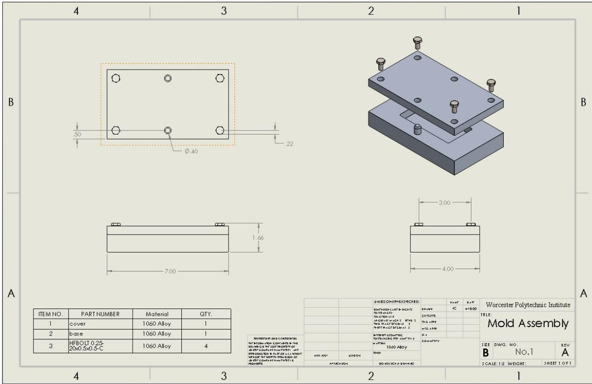
**Figure 3.2.1.** Drawing sheet for rectangular mold configuration.
