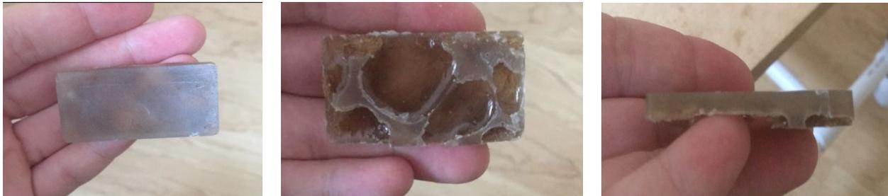
**Figure 5.1.3.** Flax-reinforced (0.5 g), hot pressed PLA sample.
