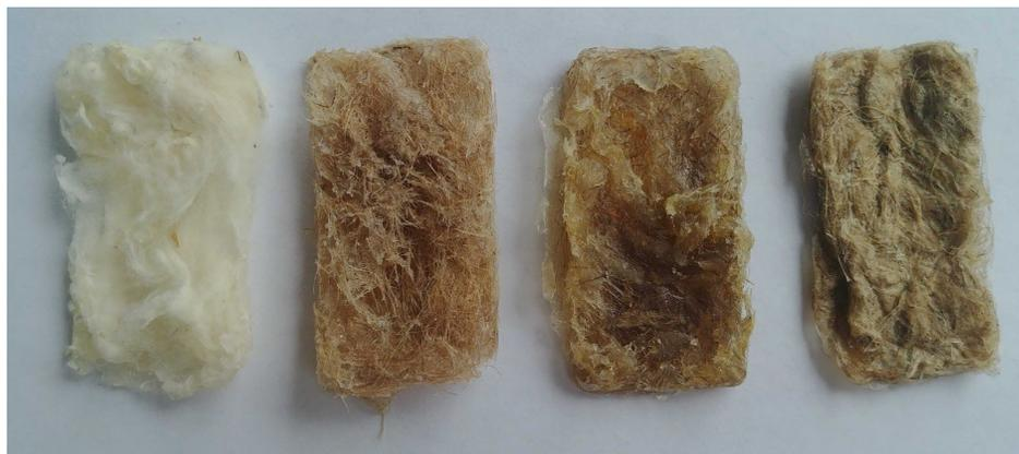
**Figure 4.9.1:** Composite samples with fiber densities exceeding the saturation limit of the matrix.
