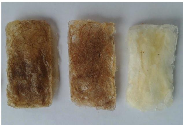
**Figure 4.4.1** Rectangular mold, Instron testable composite samples - 0.5 g flax (left), 0.5 g jute (middle), 0.5 g cotton (right).
