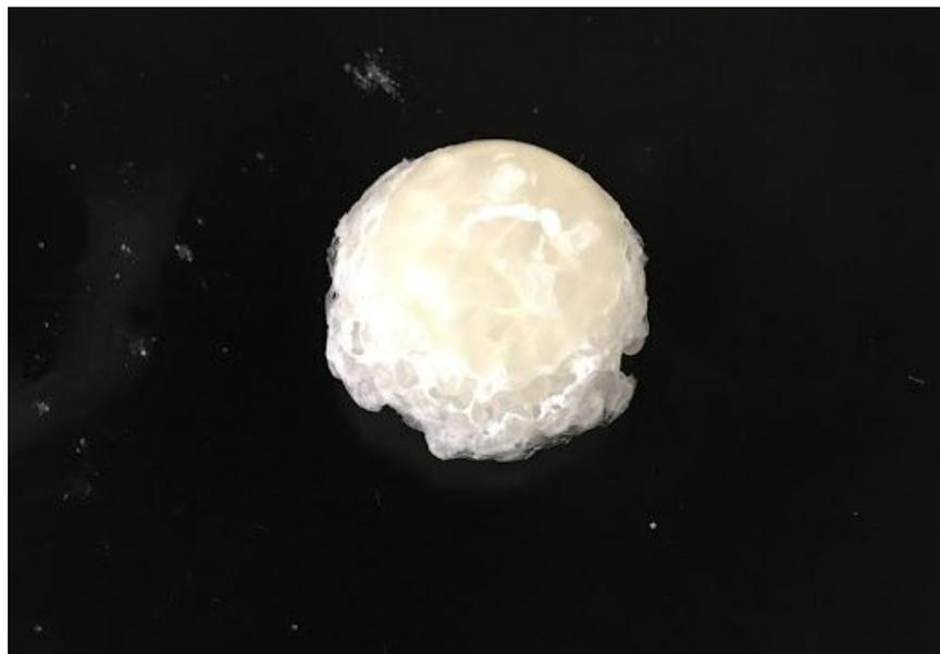
**Figure 5.1.2.** A sample of PLA pellets melted in the presence of solvents.
