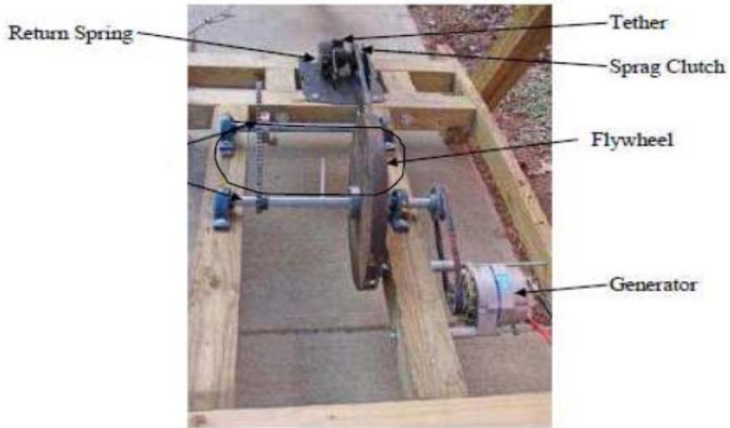
Figure 4: Generator and Flywheel on WPI Kite System
