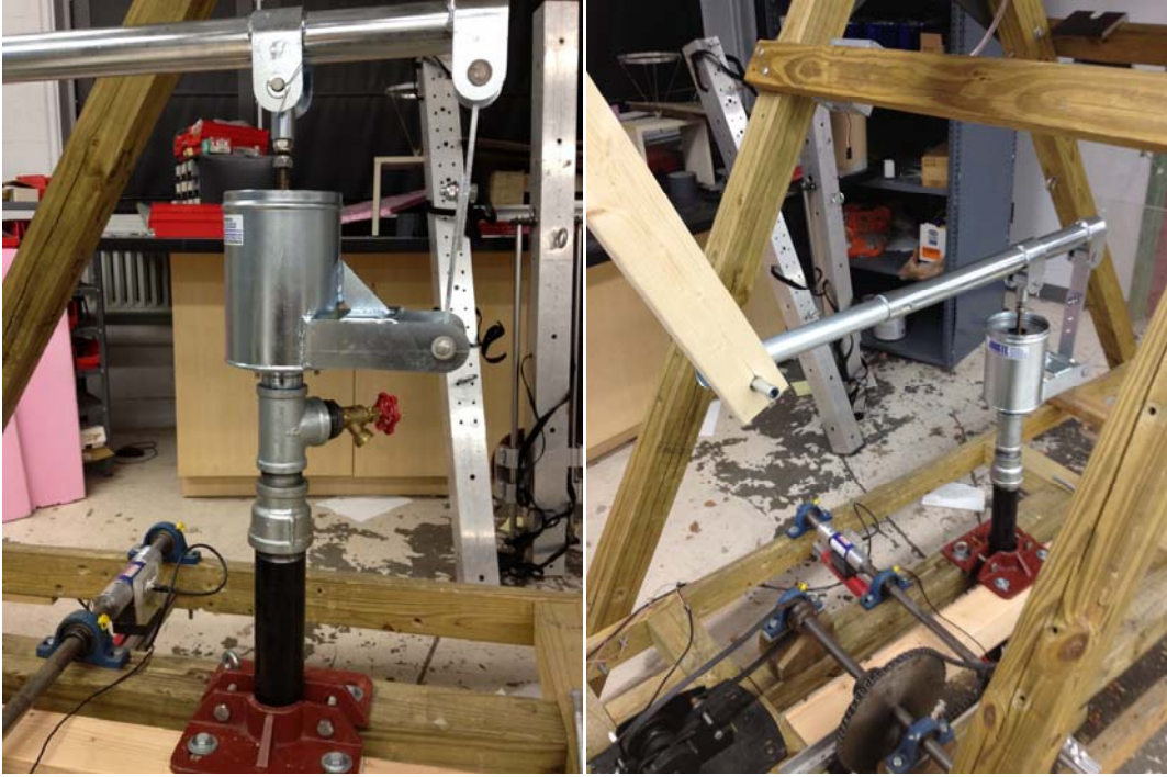
Figure 23: Pump Attached to A-Frame (Left) and Attached to Swing Arm (Right)
