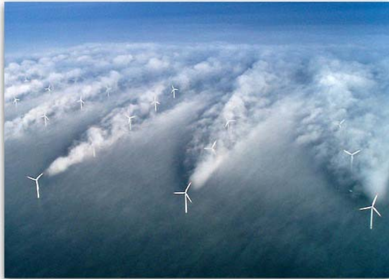
Figure 30: Turbulence Behind HAWT Horns Rev 1 Offshore Wind Turbines
