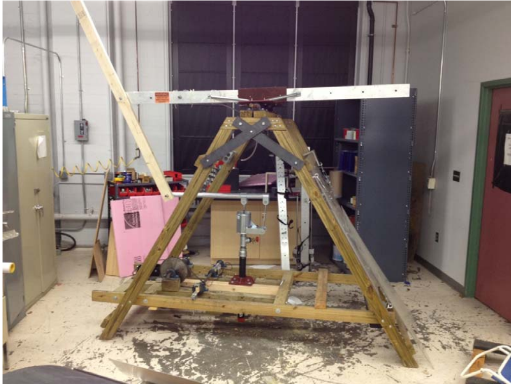
Figure 24: Pump Installed on A-Frame and Connected to Swing Arm
