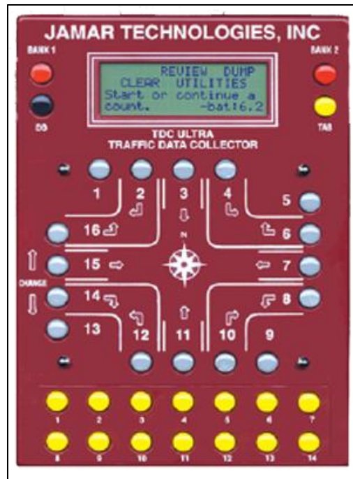
Figure 7: Turning movement counter (Jamar TDC Ultra, 2017)
