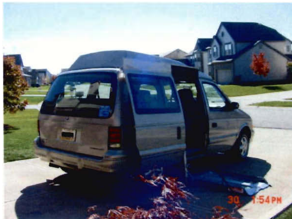
Figure 5.8: Side Hydraulic Lift (Source: Disabled Drivers' Motor Club, 2004)
