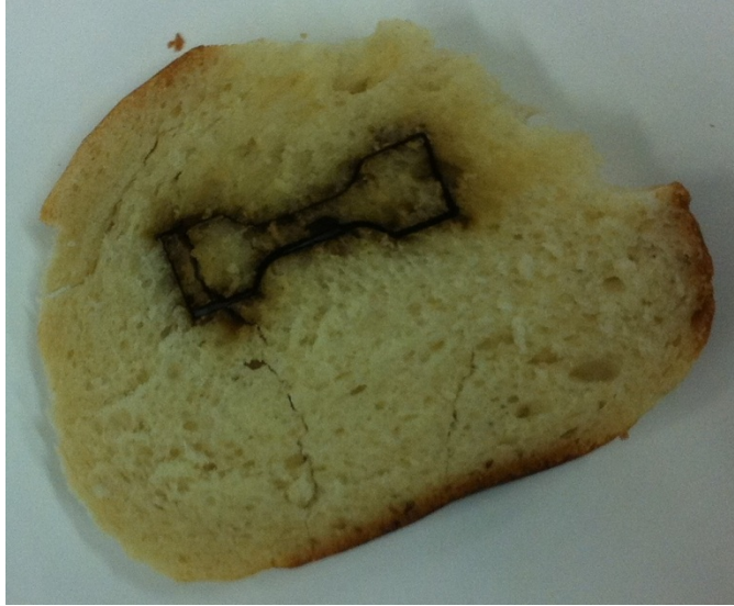
Figure 3: Tensile specimen cut out of a slice of bread, but not removed. Effect from the heat of the laser can be seen in the cut and some of the surrounding area.
