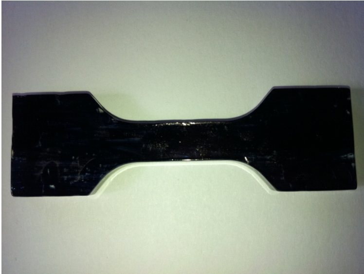
Figure 2: Sample tensile specimen cut out of 0.25 in thick acrylic.
