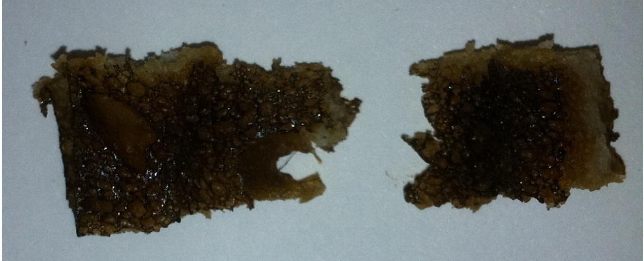
Figure 4: Fractured bread specimen showing one form of fracture. The browning caused by the heat of the laser used for cutting can also be seen, as the edge is much darker than the original color and has a shiny quality to it.
