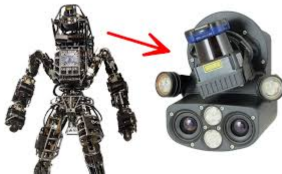
Figure 1: Atlas MultiSense head [16]
