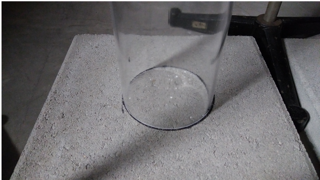
Figure 3.6: Photo of concrete base of resuspension chamber with small, white, aggregate piles of the sample dust seen in the upper right region of the enclosed area.
