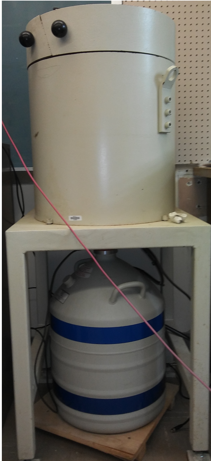
Figure 2.6: Lead-shielded Broad Energy GeLi Well Detector used to count active samples.
