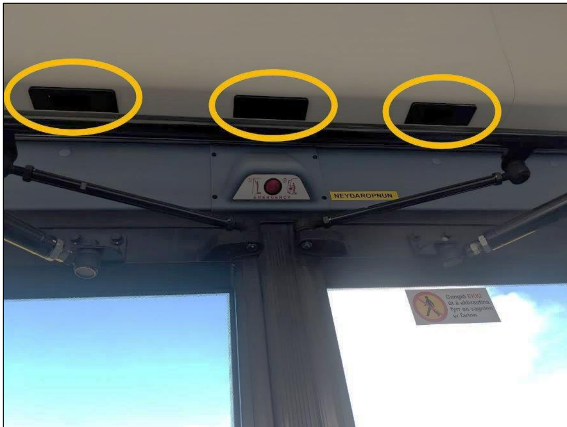
Figure 2. An image of three motion detectors (circled in yellow above the doors).
