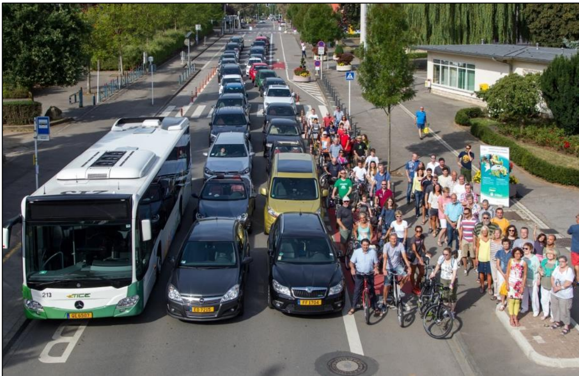
Figure 1. A comparison of the space required to transport 30 people by bus, car, bicycle, and on foot (Luxembourg Times, 2016).
