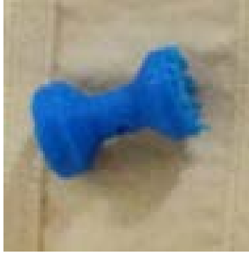
Figure 136: Failed Ratchet Mechanism System Spool
