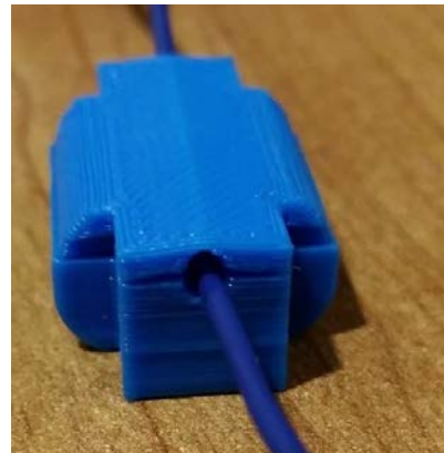
Figure 69: Gen 2 Finger; Snap Pin Failed Tolerance
