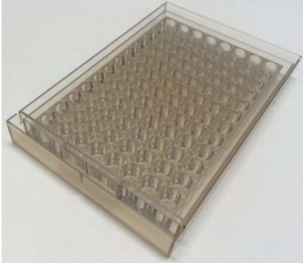
Figure 54: Final 3D Printed Prototype of Inner and Outer Plates
