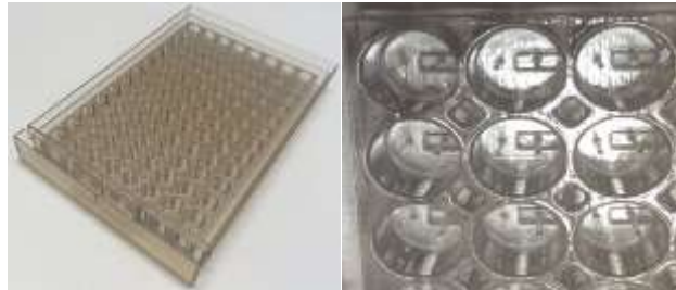
Figure 2: 3D printed prototype of top and bottom plates is shown on left, close-up of wells and posts is shown on right.
