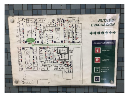
Figure 10. Evacuation sign with extraneous information that is difficult to read (By Authors)
