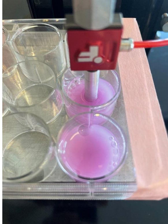
Figure 33. Fixture displacement into the acellular fibrin gel prior to recovery.
