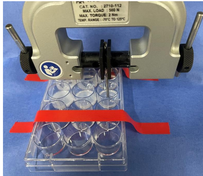
Figure 29. Instron fixture used during the first acellular indentation test.
