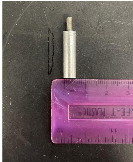
Figure 31. Final aluminum flat punch indentation fixture.
