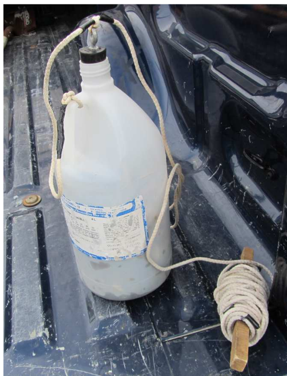
Figure 3-2: Attleboro Depth Sampler
