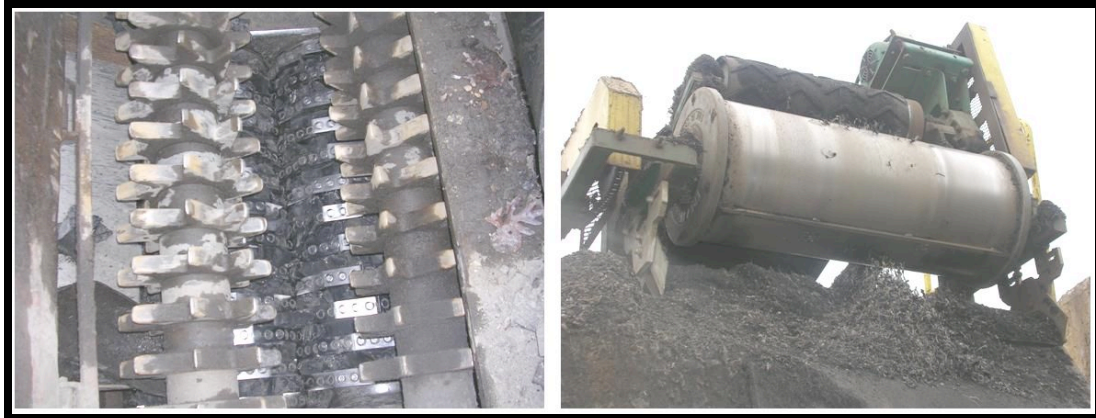
Figure 3 - Whole tyre shredding teeth on the left, and the rotating magnetic drum for separation of metal wires on the right.
