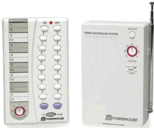
X-10 Controller (left) and Transceiver (right)
