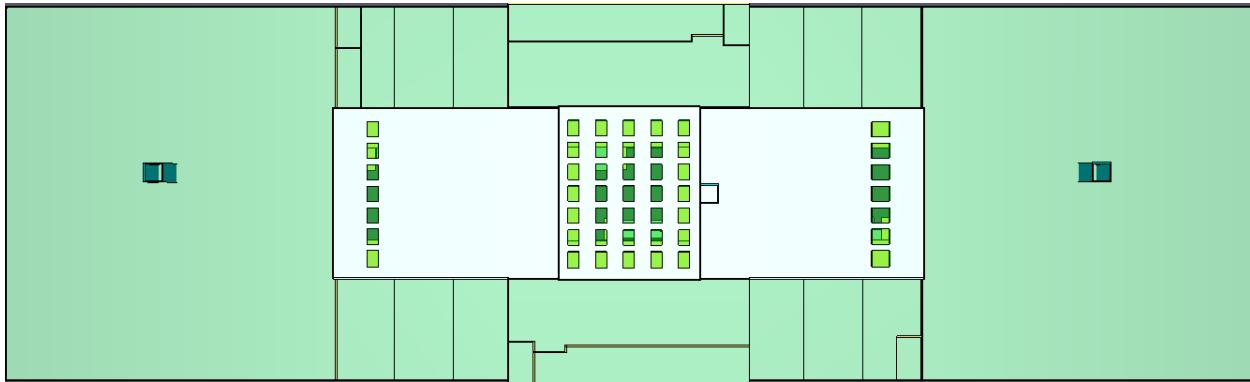
**Figure 31. Location of smoke vents in the roof and raised roof area**
