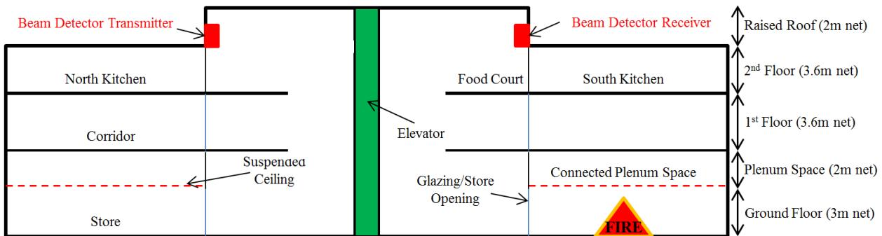
**Figure 32. Smoke detectors in the raised roof area**
