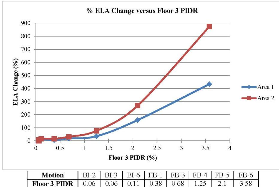
Fig. 15. Plot of % ELA change relative to 'Before BI-1' versus PIDR of Floor 3
