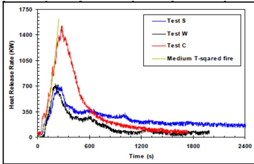
**Figure 45. Clothing store design fire HRR curve data (Zalok et al., 2007)**
