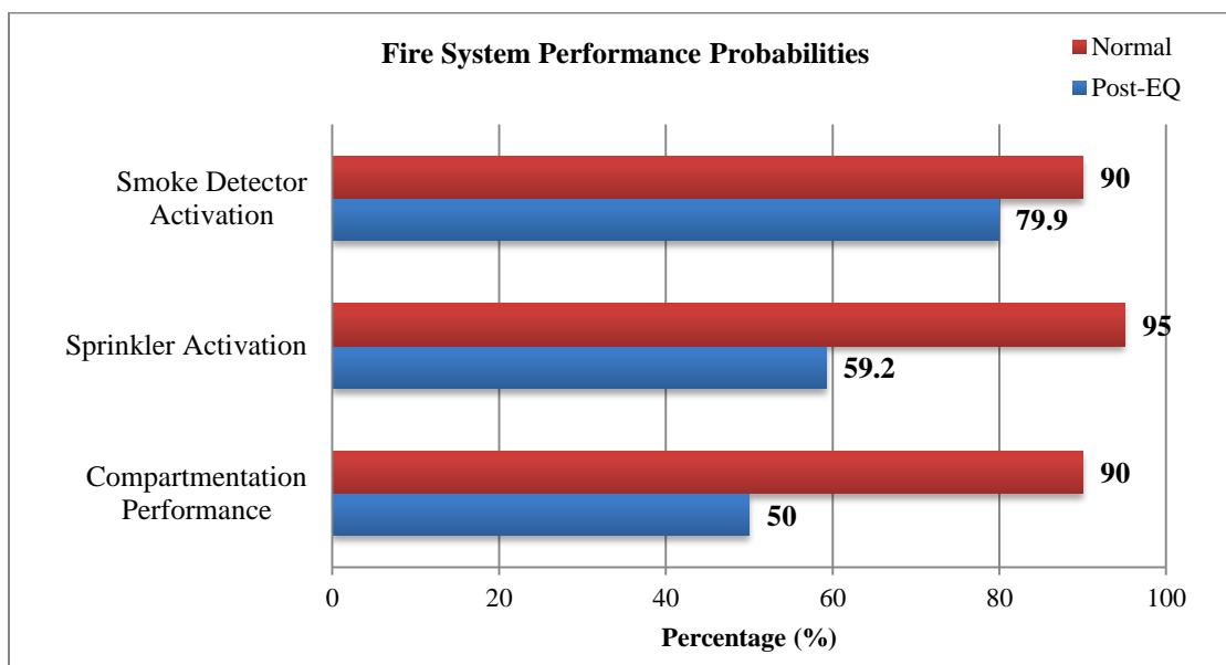
**Figure 23. Probabilities of fire system performance levels (Bukowski et al 1999; Collier 2005, Sekizawa et al 2003)**
