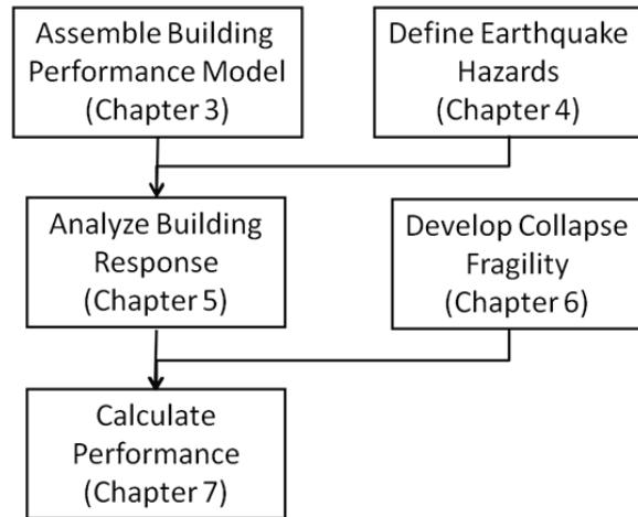
**Figure 7. ATC-58 methodology for predicting earthquake building performance (ATC-58, 2012)**
