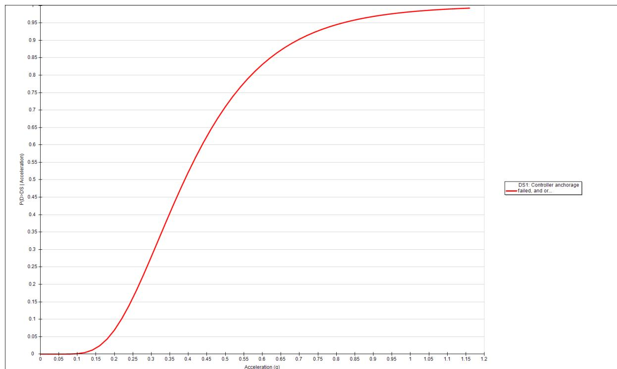
**Figure 40. D1014.011-Traction Elevator fragility (ATC-58)**
