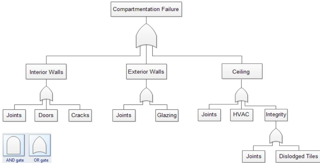
**Figure 22. Representative compartment barrier fault tree analysis**
