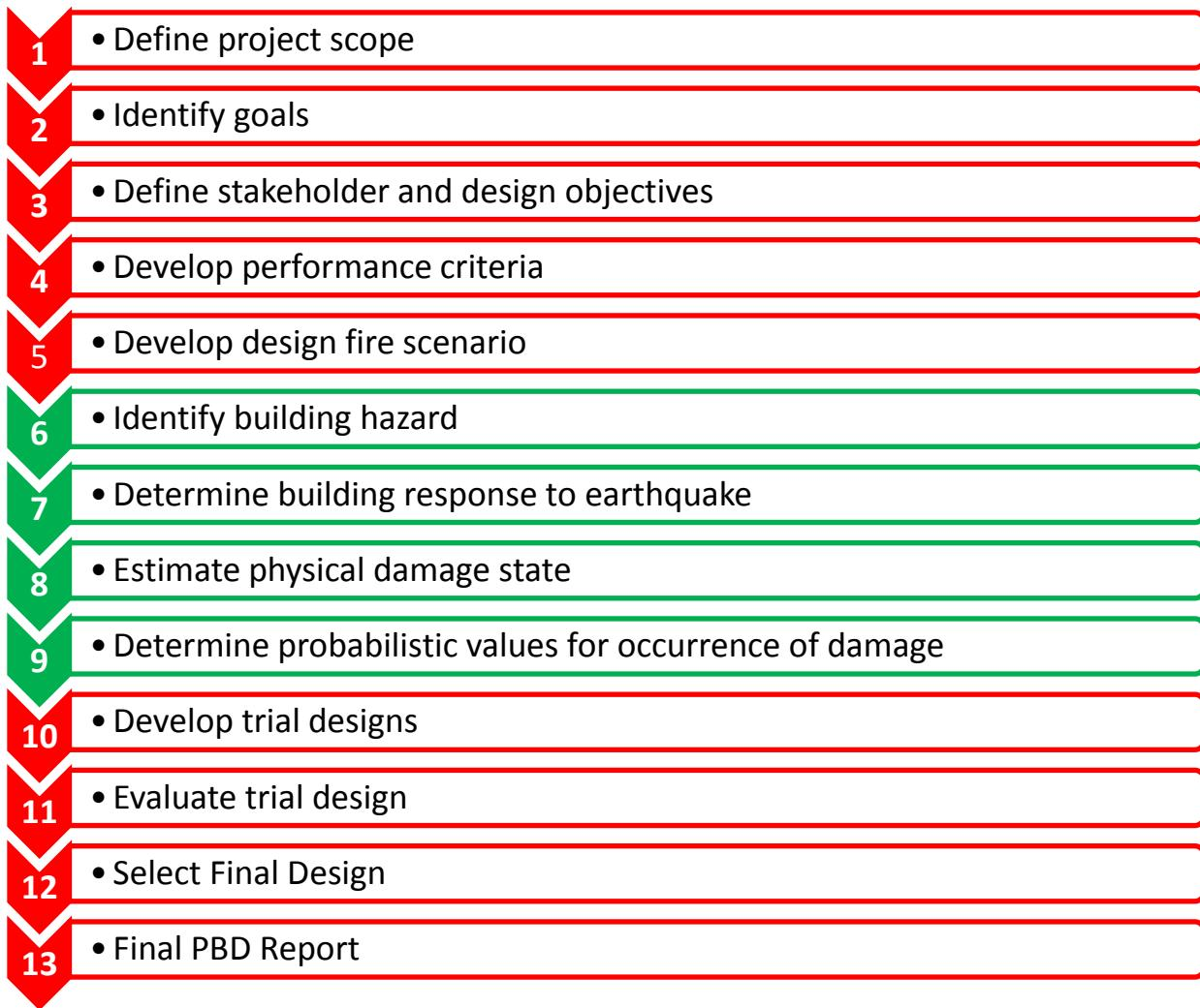
**Figure 91. Step-by-step procedure for conducting PBD on earthquake prone buildings**
