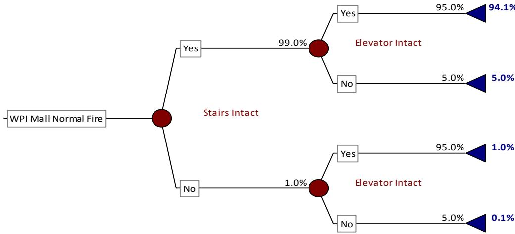
**Figure 34. WPI Mall normal evacuation event tree probabilities**
