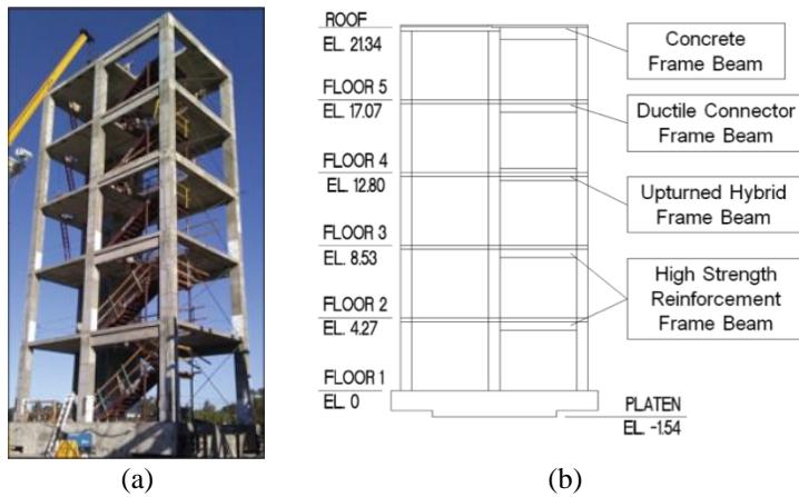
**Figure 2. Building specimen (a) skeleton; (b) elevation view (elevation in meters) [images and schematic from Chen et al. 2014].**
