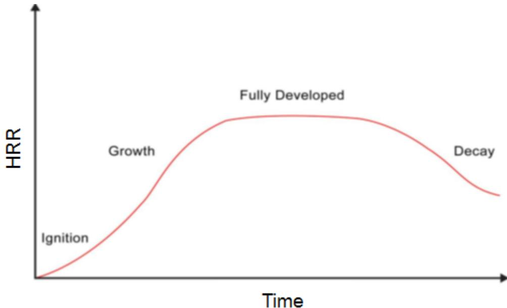
**Figure 16. Generalized fire curve**
