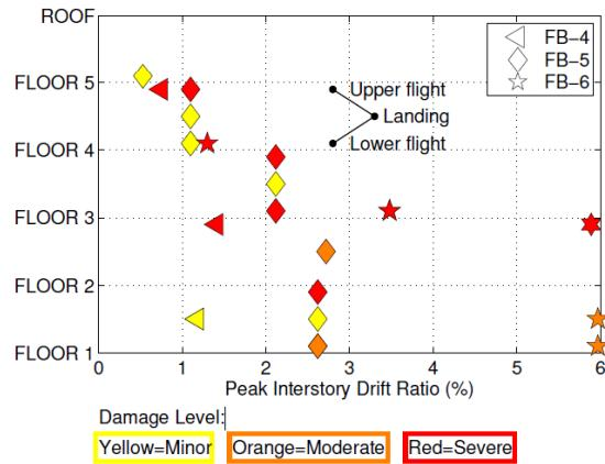
Fig. 12. Summary of damage to the stairs [figure from 13].
