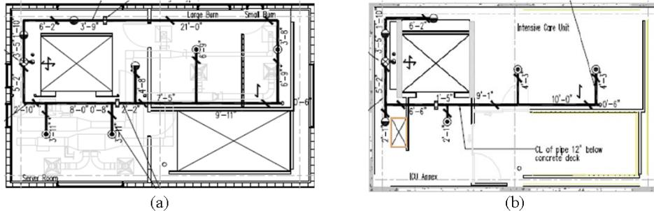
Fig. 5. Sprinkler system layout for (a) Floor 3 and (b) Floor 4 [10].
