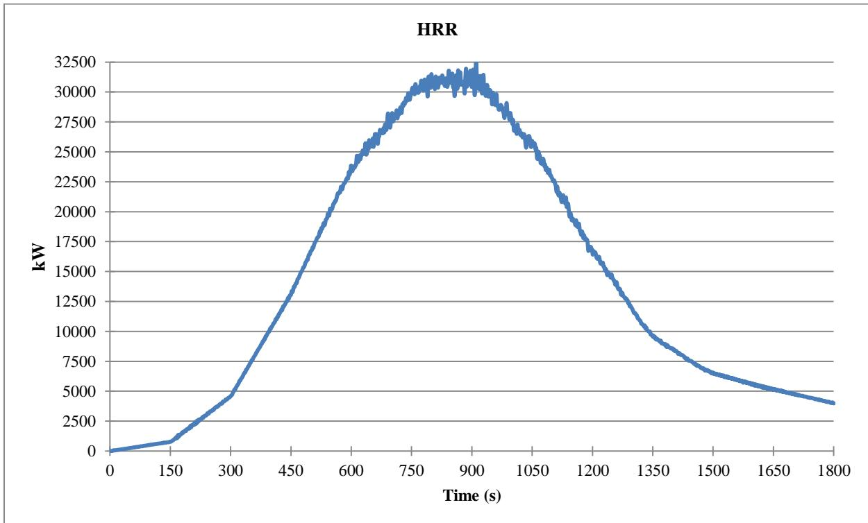
**Figure 71. Post-earthquake fire building HRR Curve**
