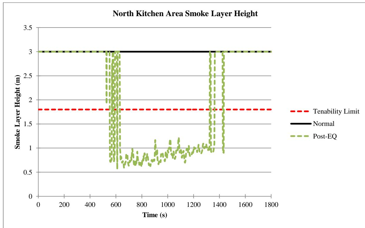
Figure 85. Smoke layer height comparison in North kitchen area
