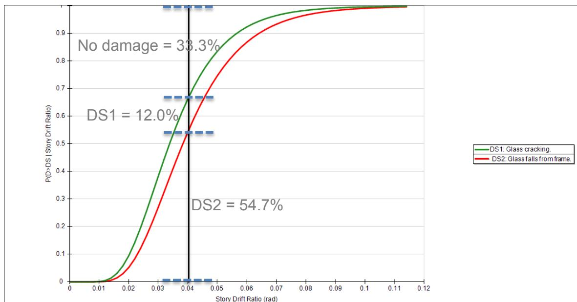
Figure 24. Fragility curve of curtain wall (B2022.001) from ATC-58 electronic database
