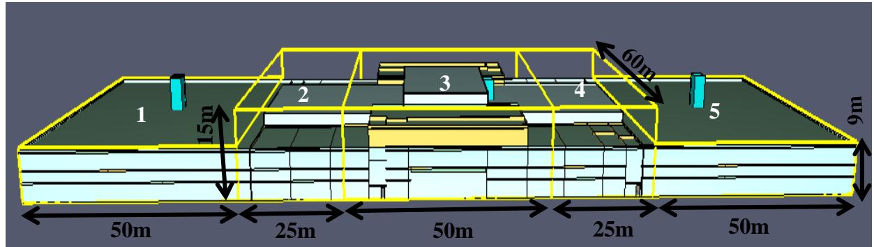
Figure 44. FDS computational domain setup
