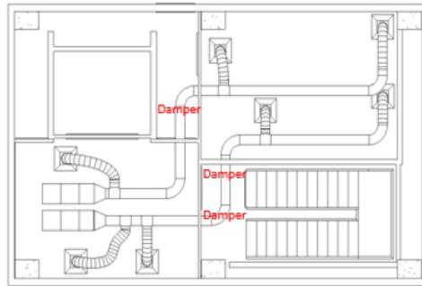
Fig. 6. Location of fire and smoke dampers
