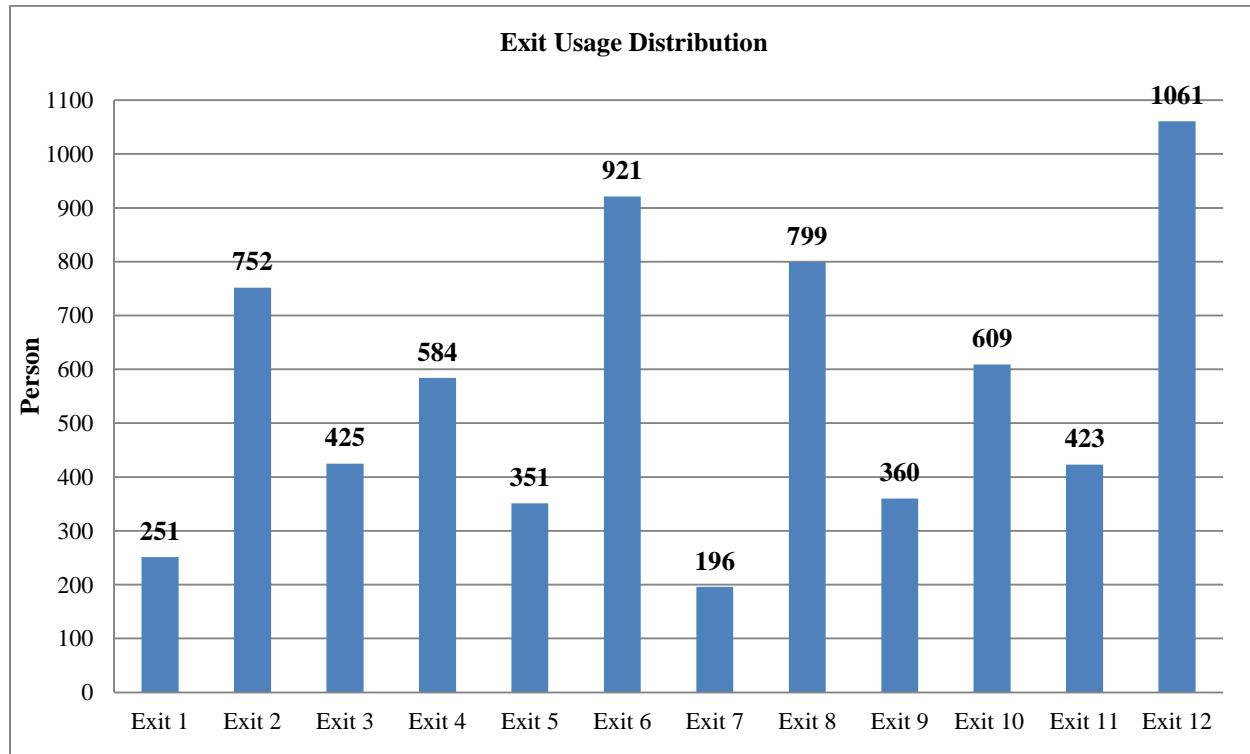
Figure 63. Number of occupant usage per exit
