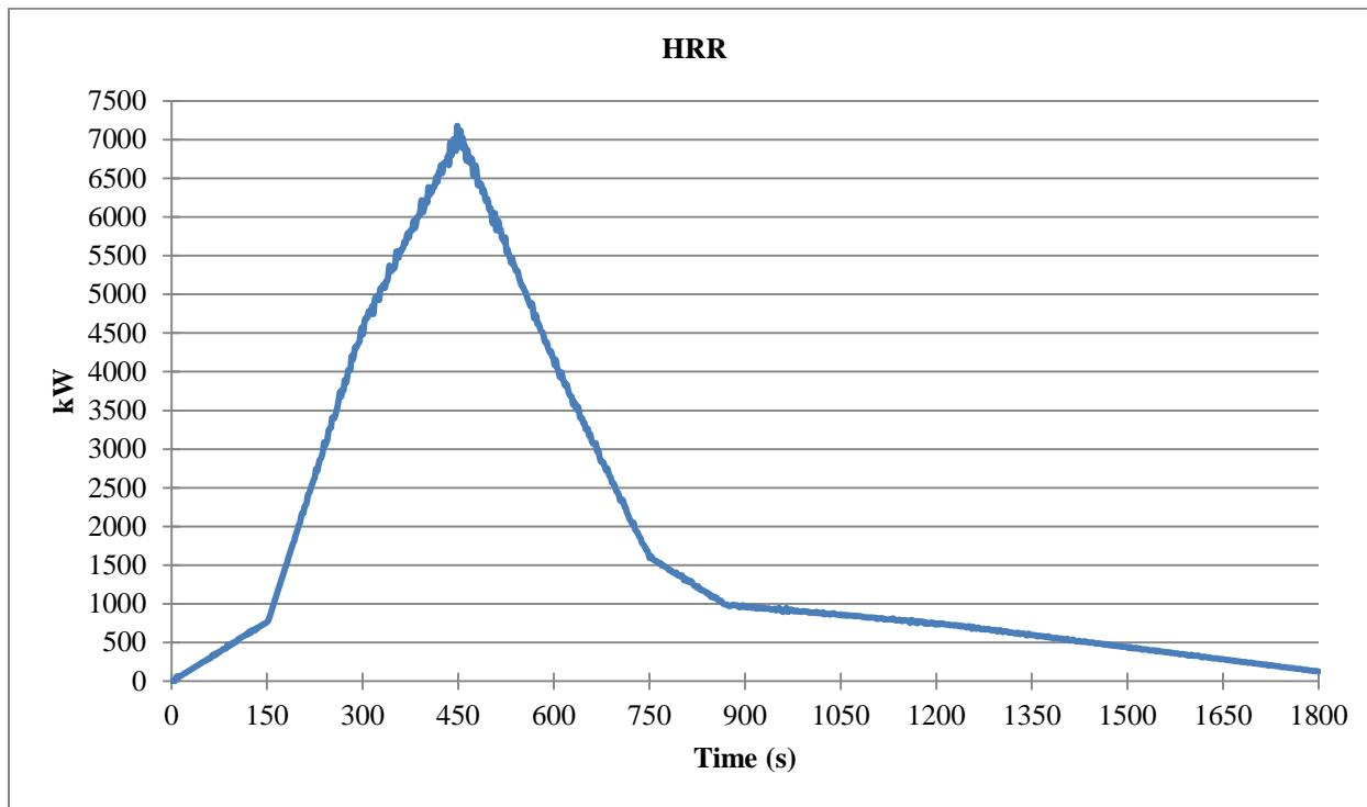
Figure 51. Normal WPI Mall HRR Curve
