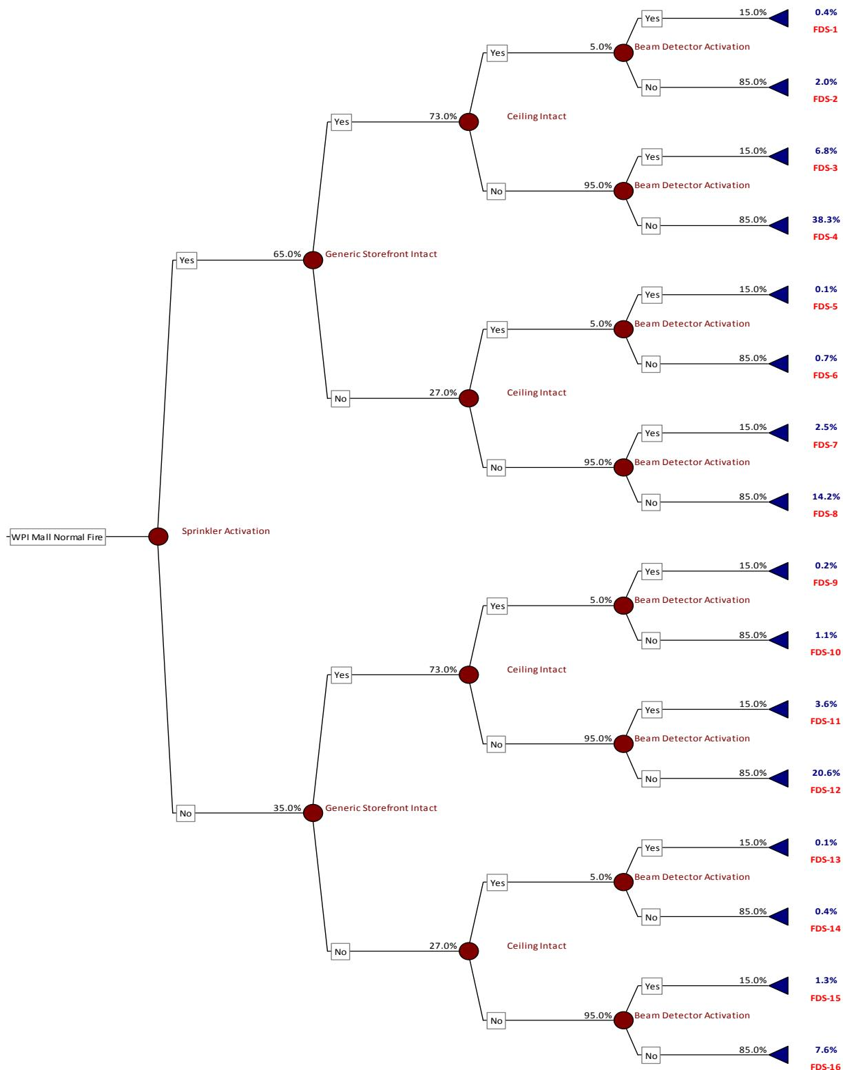
Figure 42. WPI Mall post-earthquake fire event tree for FDS modelling
