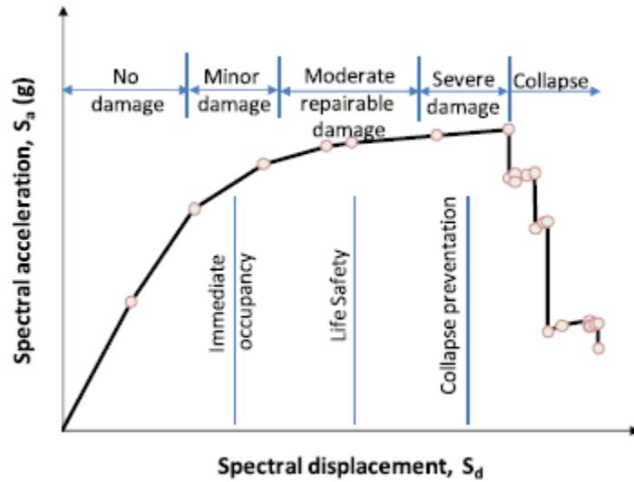
**Figure 15. Building performance with regards to earthquake response**
