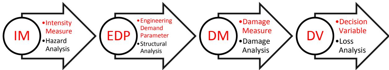
**Figure 6. PEER PBEE methodology process**
