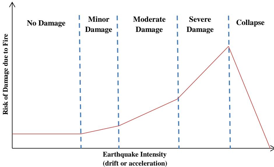
**Figure 17. Risk of damage due to fire in relationship to the earthquake intensity**
