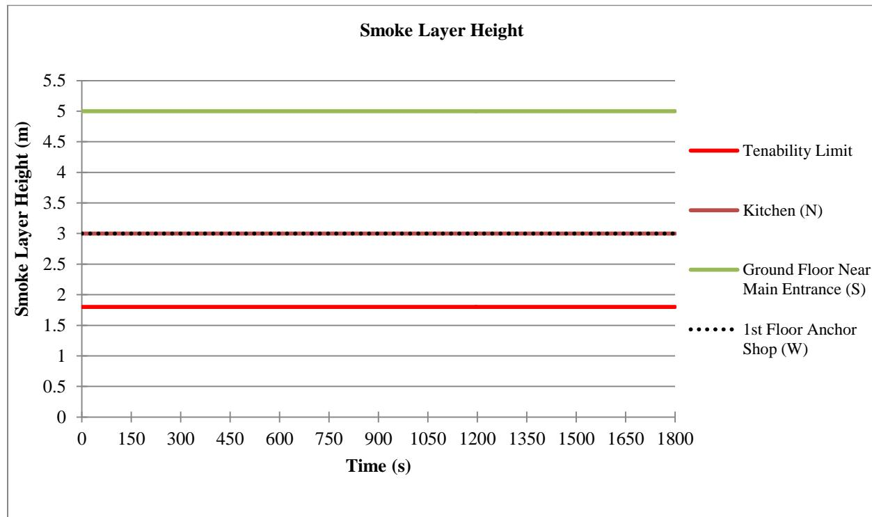
**Figure 59. Smoke Layer Heights at various locations for Normal WPI Mall**
