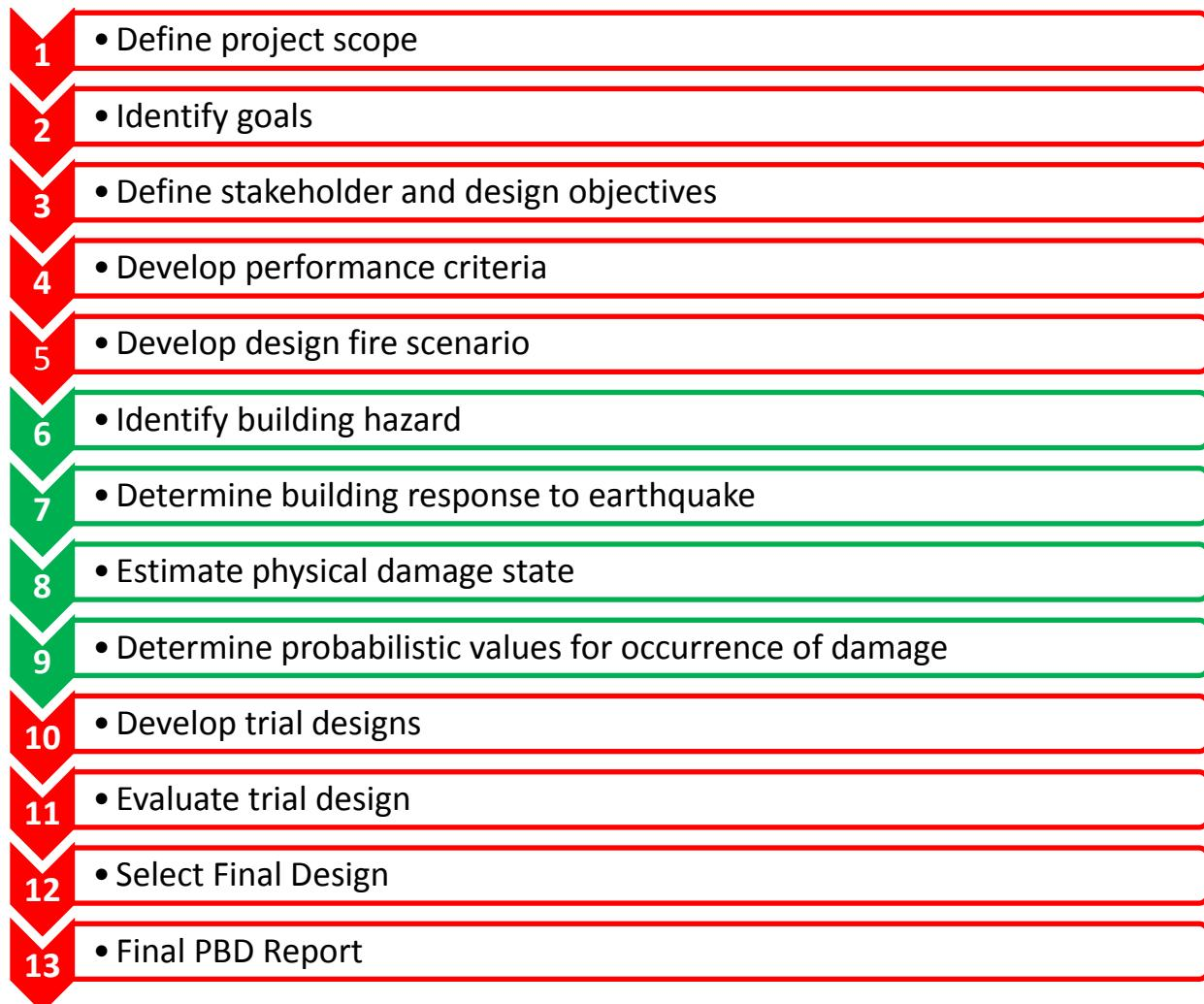
**Figure 26. Step-by-step procedure for conducting PBD on earthquake prone buildings**
