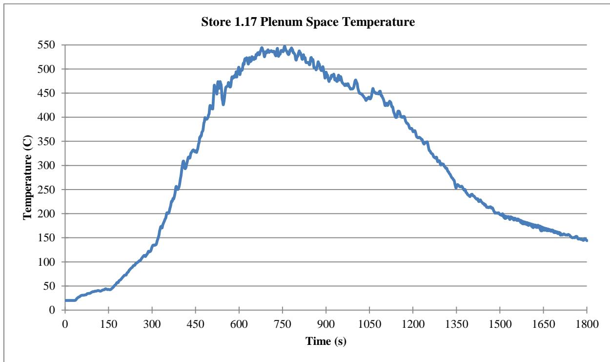
**Figure 73. Store 1.17 plenum space gas temperature**
