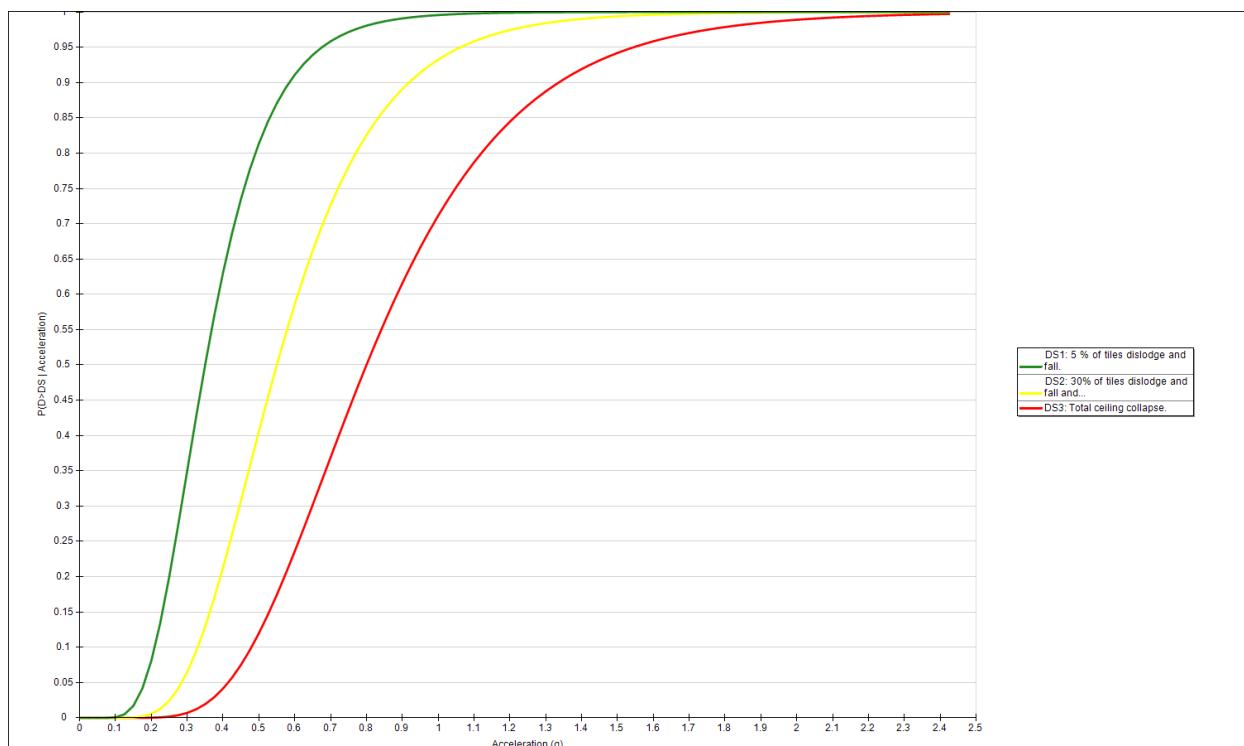
Figure 37. C3032.001c-Suspended Ceiling fragility (ATC-58)
