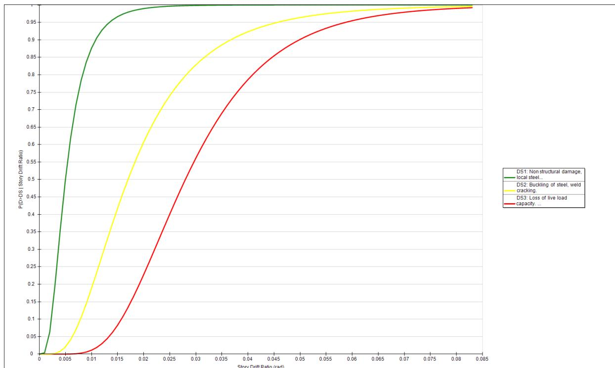
Figure 39. C2011.001b-Prefabricated Steel Stair fragility (ATC-58)
