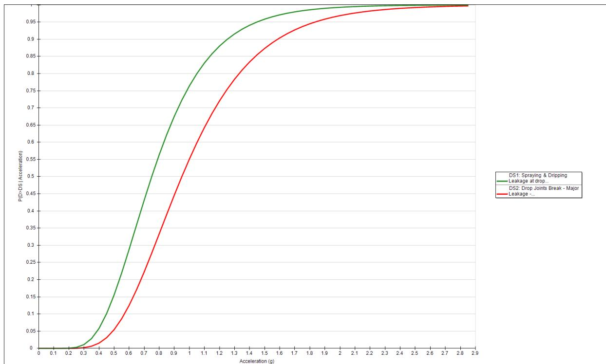
Figure 38. D4011.031a-Fire Sprinkler Drop Standard Threaded Steel fragility (ATC-58)
