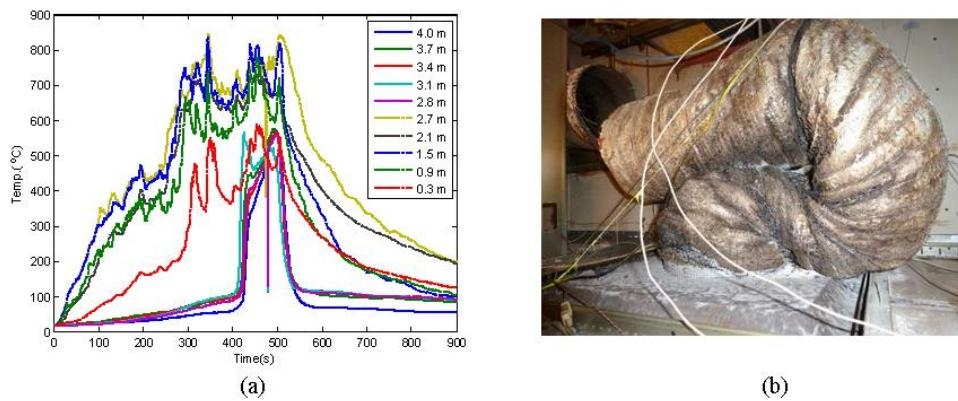
Fig. 5. Temperature increase in the space above LBR ceiling (b) and flexible duct rupture (b)
