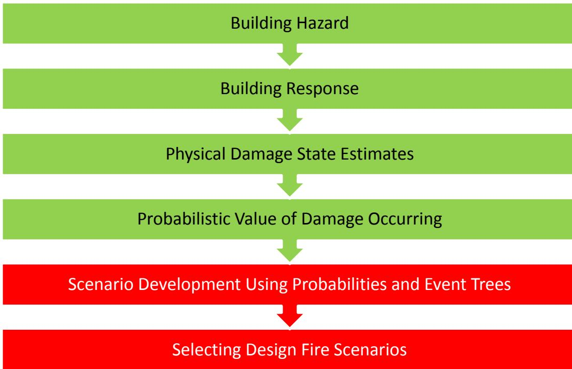
**Figure 25.** Process for developing post-earthquake building design fire scenarios
