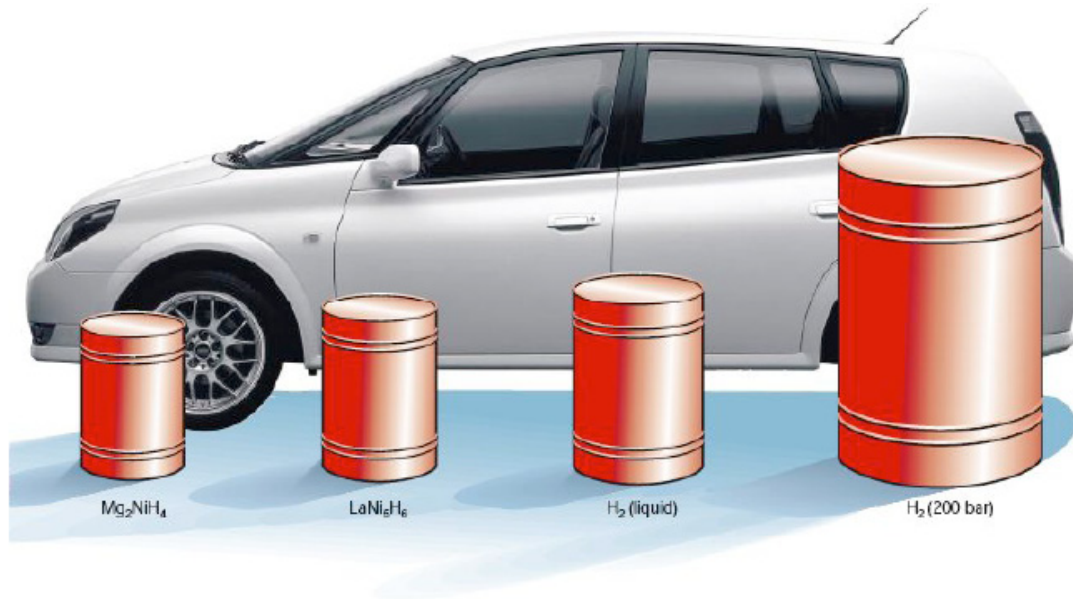
Figure 1-2: Volume of 4 kg of hydrogen compacted in different ways, with size relative to the size of a car [3].
