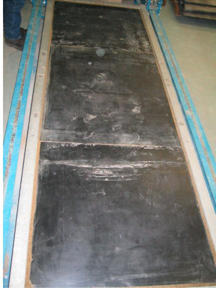
Figure 9.3: Compaction platform with neoprene layer for trial slab
