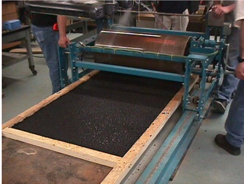
Figure 6.2: Compaction of HMA in the mold using vibratory compactor
