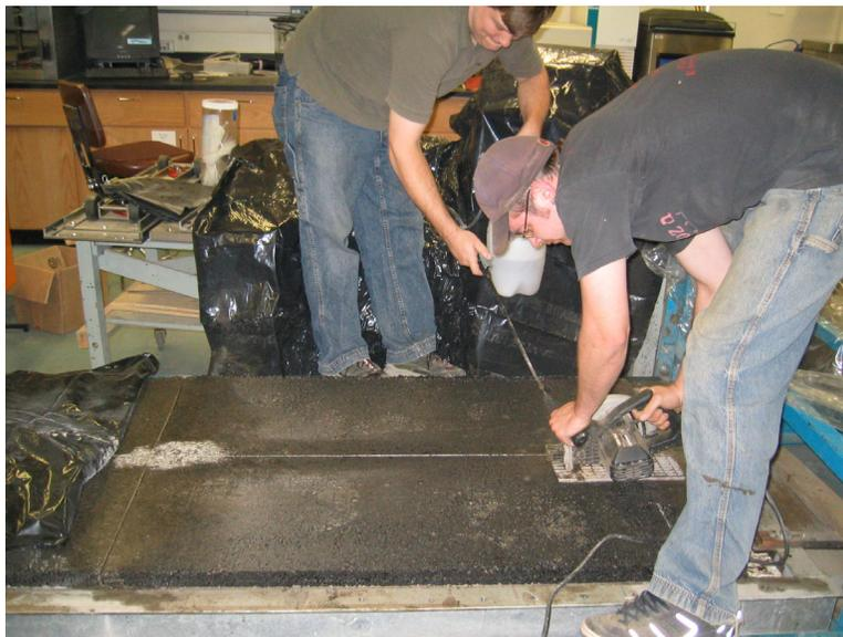
Figure 9.13: Cutting of slab after cooling by dry ice (note dry ice bags on top of adjacent slabs)
