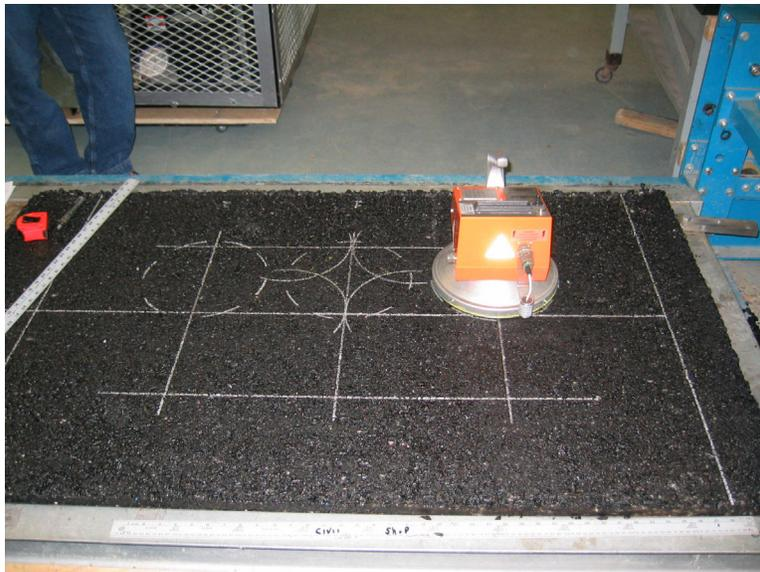
Figure 9.12: PQI readings are being taken on top of the compacted slab
