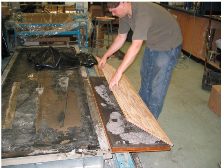
Figure 9.15: Sliding slab onto plywood board.
