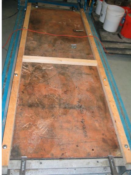
Figure 9.5: Steel compaction platform with wooden frame
