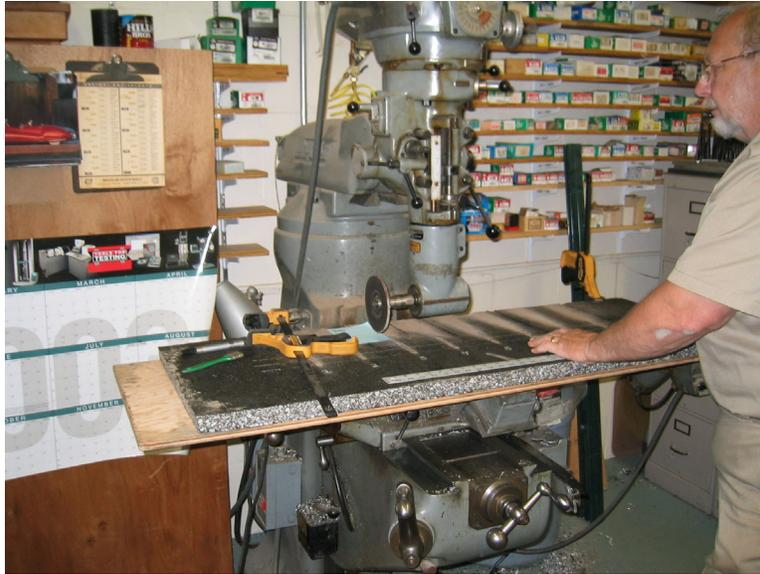
Figure 9.17: Cutting grooves for strain gauges and thermocouples
