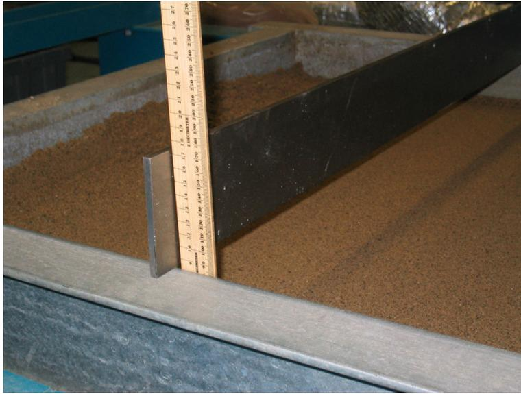
Figure 9.2: Leveled surface of sand
