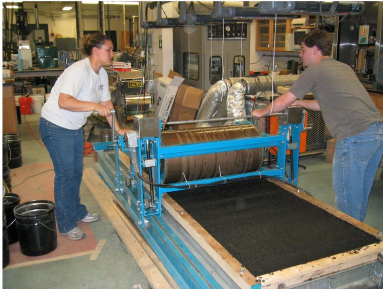
Figure 9.11: Compaction of HMA in the mold
