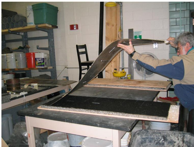
Figure 9.7: Aluminum sheets were peeled off from bottom of test slab
