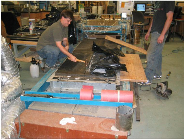
Figure 9.14: Separating slabs.
