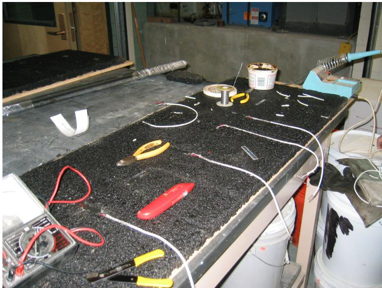
Figure 9.18: Attaching strain gauges
