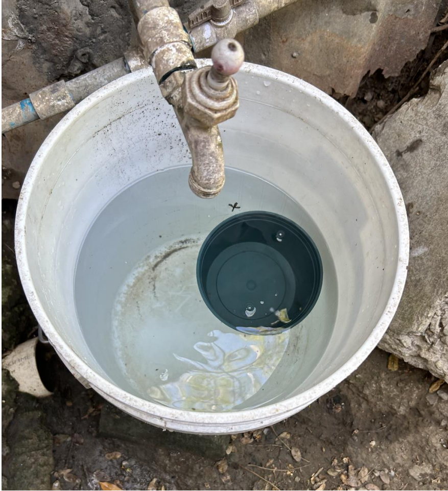
Figure 14: 5-gallon Holding Bucket in La Libertad showing visible sediment and bugs present in the water (tested positive for E.coli )
