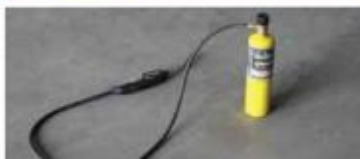
Figure 30: A hose extension added to a blow torch.
