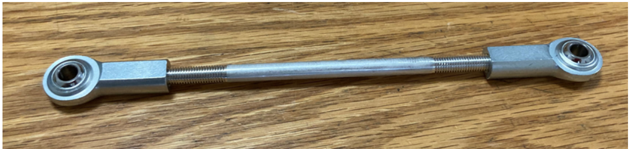
Figure 23: Ball Joints (12) and Connecting Rod (13)
