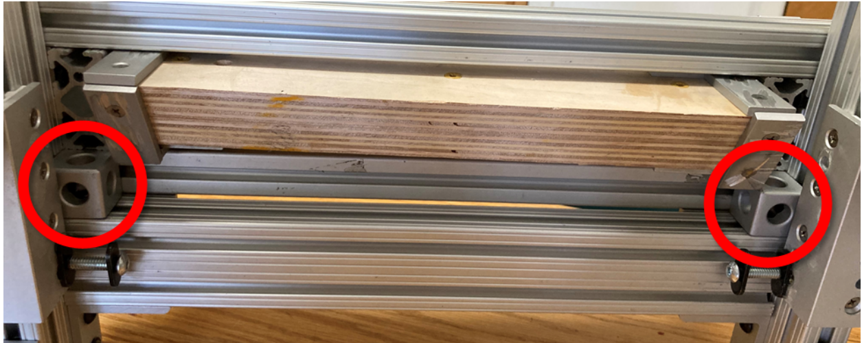
Figure 36: 3-way joints that connect the wedge housings to the frame
