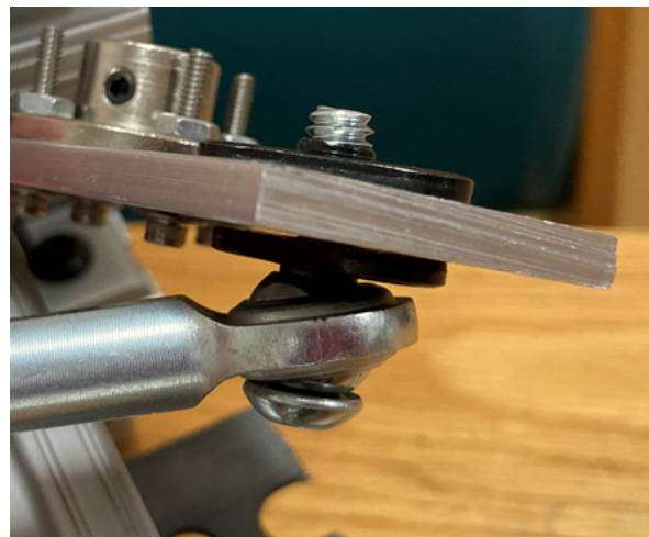
Figure 25: Joint between Linkage Arm and Crank Arm
