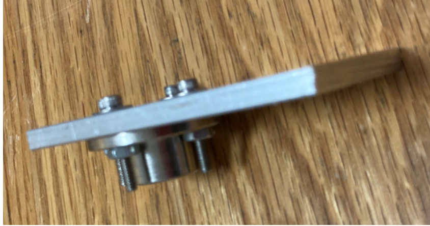
Figure 24: Crank Arm (14) and Crank Hub (15)
