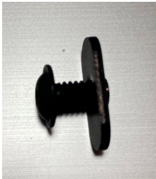
Figure 15: 1/4" -20 fastener and elongated nut used for 80/20 components
