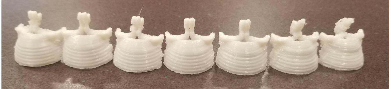
Figure 5.19: Printed eyelids - layer heights 0.06 to 0.6 mm from left to right
