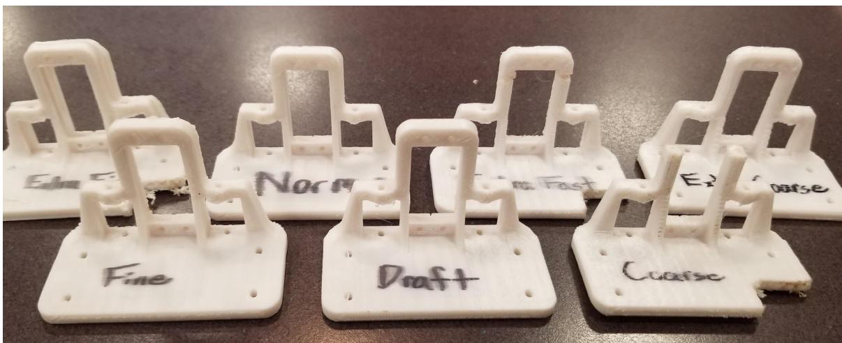
Figure 5.20: Printed servo mounts - layer heights 0.06 to 0.6 mm
