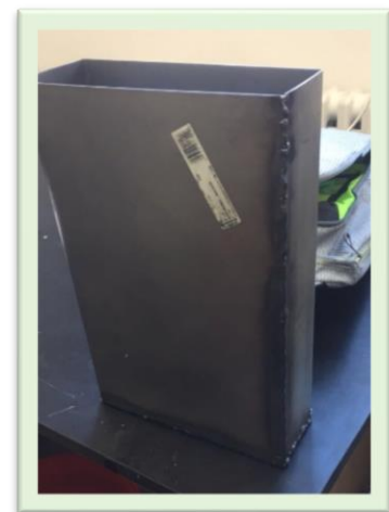
Figure 4: Metal box created to make mold of 3D flipper in.
