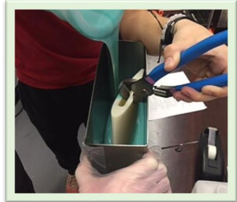
Figure 5: Holding the 3D printed flipper in place while the mold mixture is poured around the flipper.
