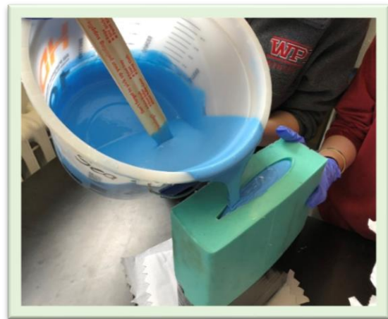
Figure 7: Pouring the Smooth-Sil 950 into the mold
