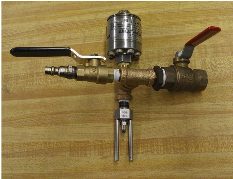
Figure 21: The Valve and Gage Used to Calibrate the Pressure Transducer
