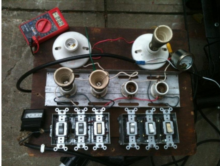
Figure 16: Circuit Board Used for the Dynamometer Test Performed on the NorEaster Engine
