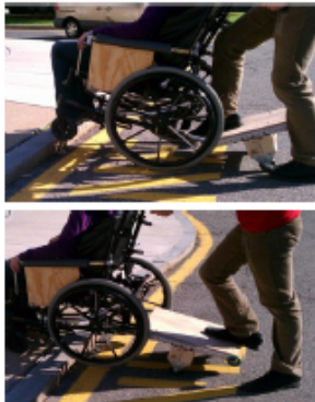
Figure 1. Operation of the wheelchair lifting device seen lifting the front and rear wheels of the chair.
