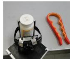
Figure 7. Prototype device used to stabilize the jar pictured on the left next to an existing product used to grasp the lid.
