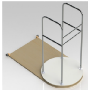
Figure 3. The rotating walker device to assist persons arising from a bed is seen as modeled using Computer Aided Design.
