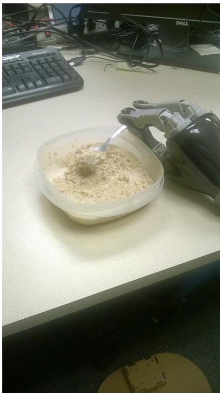
FIGURE 4.6: Optimal end-effector grasp pose for self feeding task
