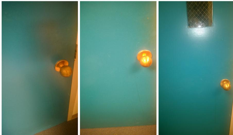
FIGURE 3.4: The change in reflectivity at varying lighting condition. Left: Environment with dull light Centre: Environment with bright light Right: A subset of door points having brighter intensity than the handle causing noise
