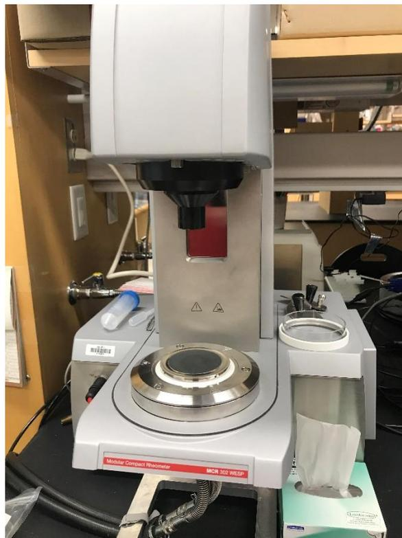
*Figure 26: MCR 302 WESP Rheometer Used for Testing Hydrogel Stiffness Properties*
