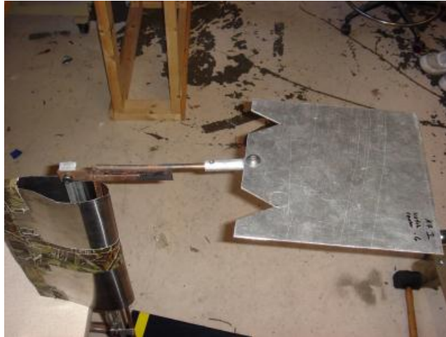
Figure 22: Force Balance Stand with Drag Shield
